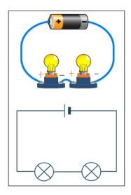
In a Series circuit, if a fault occurs at one point, the total circuit will break and all the components are arranged in a single line.
