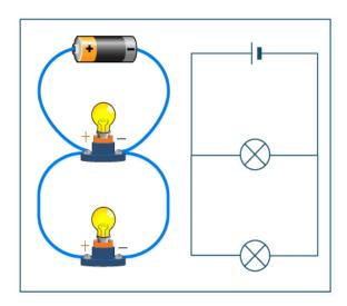
In a parallel circuit, if any one component gets damaged, the current does not stop and continues to flow through the other components; hence other components work efficiently and all the components are arranged parallel to each other.
