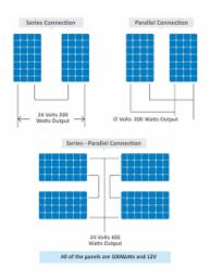
Solar panels are wired in series to increase the voltage in order to meet the minimum operating requirements of the inverter. If solar modules are wired in parallel, the positive
