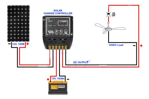
Solar fan is can be easily bought from the market, it is a DC fan which can be used on the Solar energy. When Light Falls on the PV modules generate electricity (DC Current), Which can be directly used to run DC fan.
